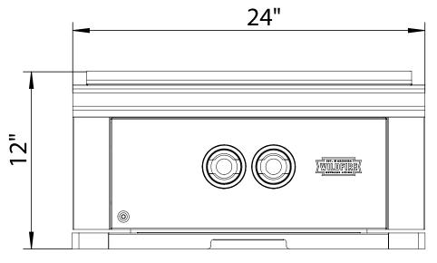
Slide-In Power Burner WF-POWBRN-RH-NG/LG
