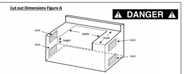
Minimum of 2 vents, but optimally 4 vents, per cabinet that has any sort of gas supply or connection. Each vent must be at least 20 sq inch in size and have access to outside/fresh air.
